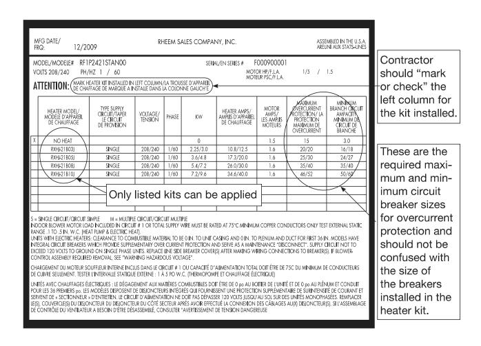
Heater Kit Supplemental Information: What allows the manufacturer to use standard Circuit Breakers up to 60 amps inside the air handler, when using an approved Heater Kit?
