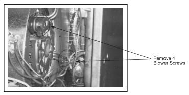
12. Lower the blower and turn assembly counter clockwise with the motor pointing towards the top of the air handler.
