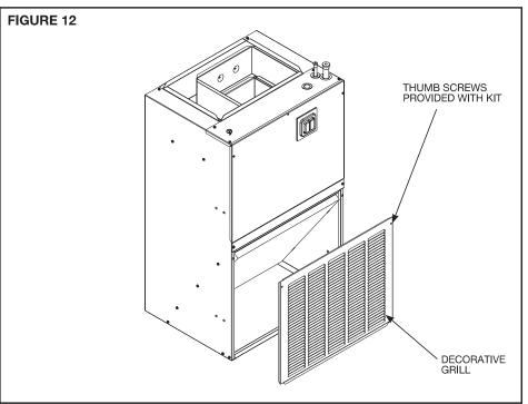
**6.5 DECORATIVE WALL GRILLE Decorative Wall Grille RXHK-D01/RXHK-D02** is used in applications where the air handler is installed in a closet or interior wall and allows adequate return air back to the unit.
